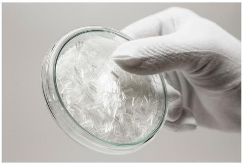
Quartzel<sup>®</sup> fiber is a homogeneous, non-porous, continuous, amorphous, ultra-pure silica glass with a SiO<sub>2</sub> content  $\geq$  99.95%. Quartzel<sup>®</sup> chopped strands are produced from either 9µm or 14µm Quartzel<sup>®</sup> rovings which are chopped to a pre-determined length.
